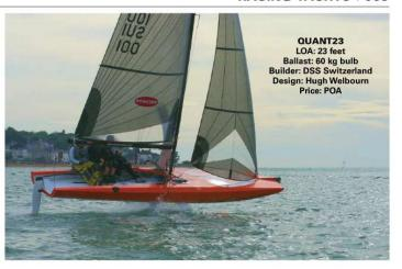
The Quant 23 proves that foiling systems are reaching a new level, which could radically change racing in the near future.
