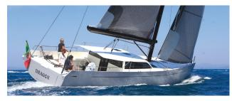
ast in all conditions, with a large and well protected cockpit, 360° panorama deck salon, two engines for maximum reliability and easy maneuvering, large dinghy garage. Built in E-glass multiaxial fiber and epoxy sandwich with structural reinforcements in carbon fiber. A great Bluewater yacht to sail shorthand in all conditions, with highest standards of safety and performances.
