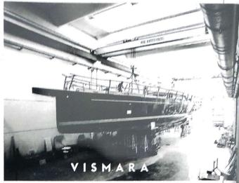
A carbon composite hull brings the V100B in at just 62 tonnes
